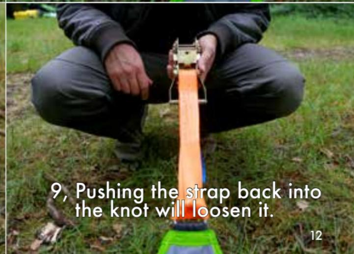
9, Pushing the strap back into the knot will loosen it.
