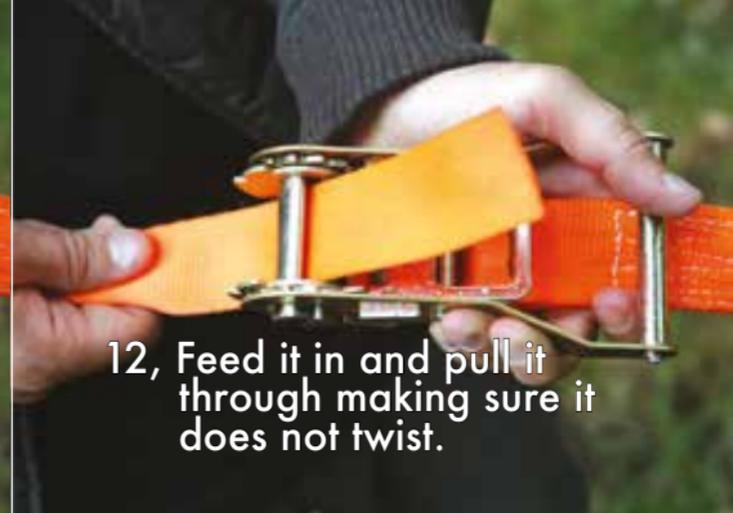
12, Feed it in and pull it through making sure it does not twist.
