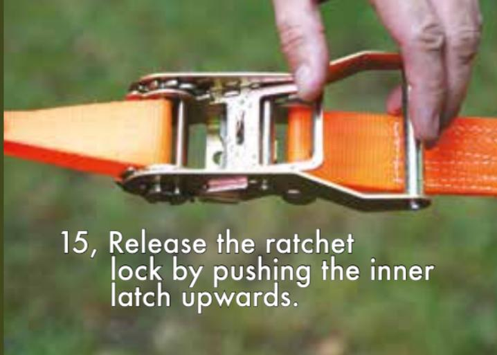
15, Release the ratchet lock by pushing the inner latch upwards.
